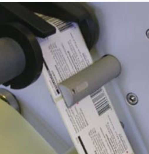
◀ Automatically adjusted sensor adjusts itself by label change
