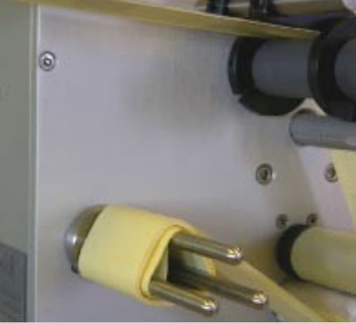
◀ Reeling with room for a whole roll of liner
